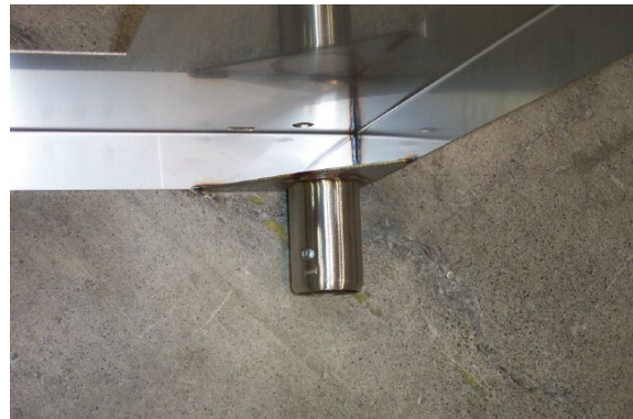
Figure 1—Leg socket showing set screw
